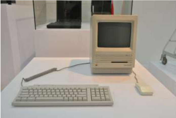
Photo 8: The iconic Apple Mackintosh piece was designed in 1987 under the Snow White design concept, setting the new tone and attitude characterised by pronounced clarity with regards to the radii of the curves, the inlaid logo without a border, and the product labeling.
